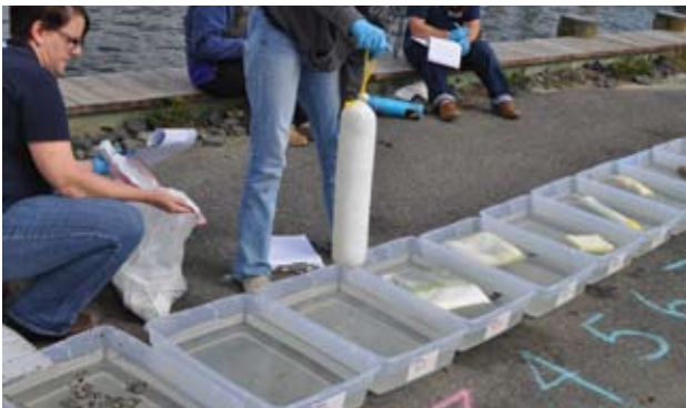
Photo Caption: In addition to Duke University Marine Laboratory testing, the BoatUS Foundation also attempted to simulate the use of oil spill products in the bilge.
